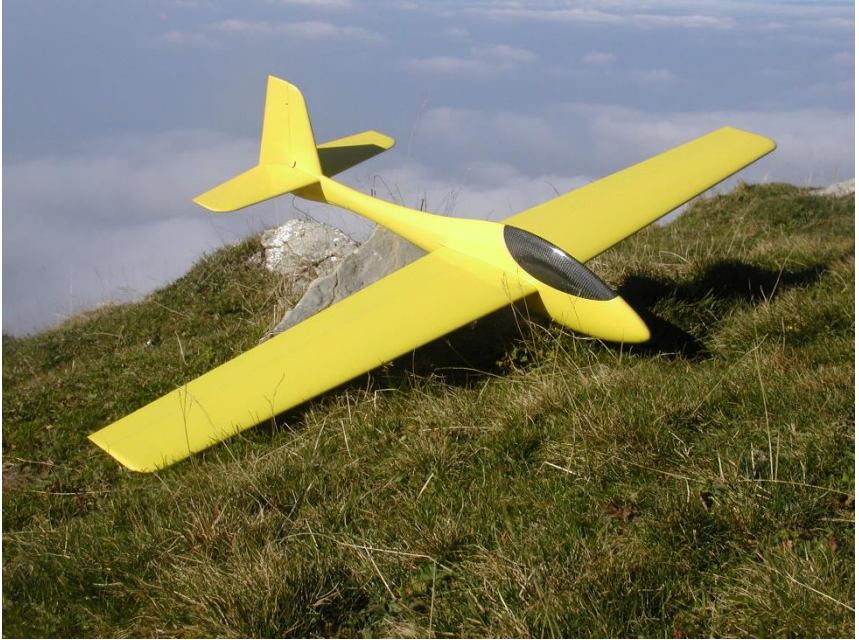
The Wasabi is an aerobatic glider, designed by Thierry Platon, Jérôme Bobin and François Lorrain, which benefits from an in-depth study of the fuselage for the phases of knife-edge flight (photo Jérôme Bobin).
