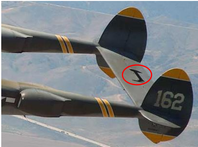
Fig. 109, anti-flutter mass (elevator rudder, Lockheed P38).
