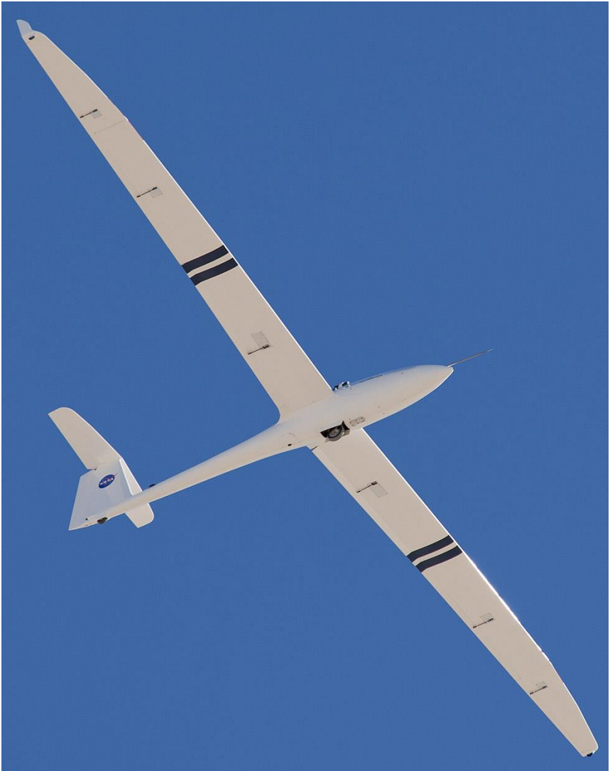
A significant aspect ratio is, far more than the airfoil, the secret to the efficiency of sailing machines (NASA photo).
