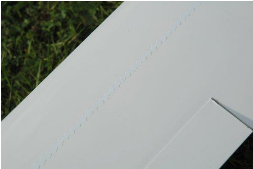
Fig. 91: Example of a zigzag turbulator on a DG1000 wing
